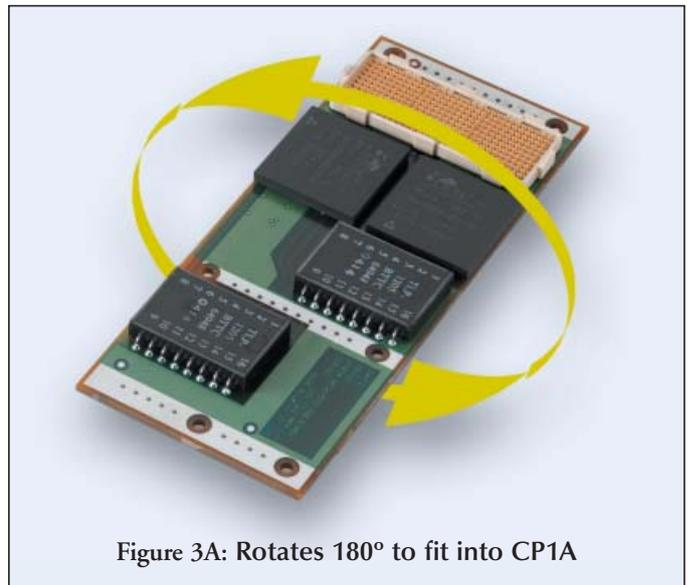
Figure 3A: Rotates 180° to fit into CP1A
