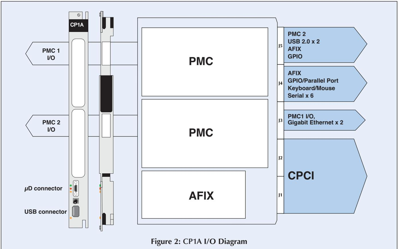
Figure 2: CP1A I/O Diagram
