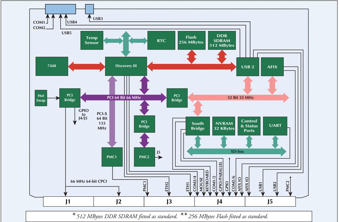
Figure 1: CP1A Functional Block Diagram
