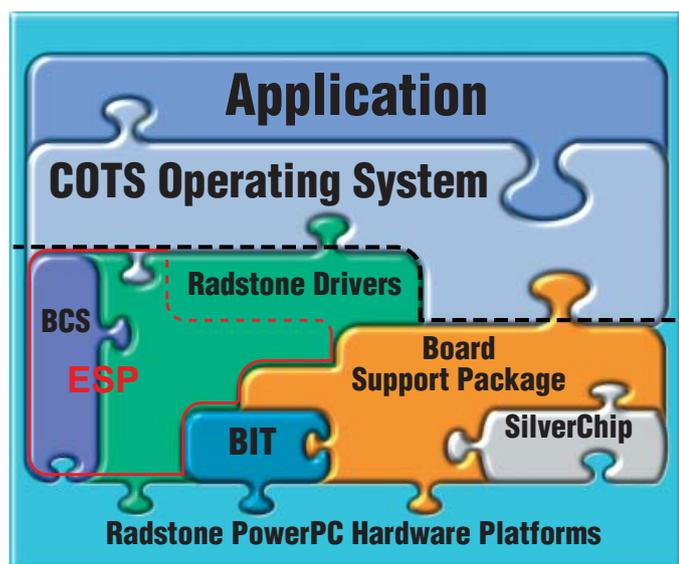
Figure 4: Software Support Model
