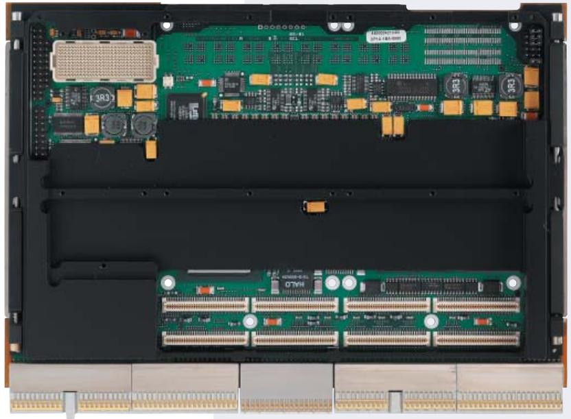
The CP1A 6U CompactPCI single board computer (SBC) is the founder member of Radstone's brand new PowerPact6 family, building on the success of Radstone's established PowerPact3 family of 3U CompactPCI products.
